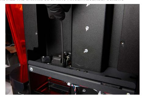
Place the three 2 mm hex screws into their respective holes in the cartridge spring finger assembly and thread them into the floor of the cartridge slot. Tighten the three screws using the provided 2 mm hex driver. Do not overtighten to avoid stripping the screw threads.
