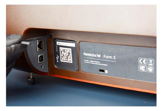
Rotate the printer to access the rear. Use the provided 3 mm hex driver to loosen and remove the two screws on the back of the printer, near the power and data ports.
