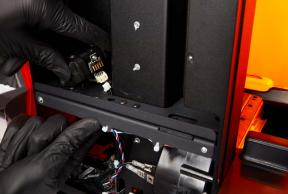
Gently lift the cartridge spring finger assembly away from the bottom of the cartridge slot. Locate the cartridge spring finger assembly cable. Hold the connector by its plastic housing and disconnect the cable from the cartridge spring finger assembly board. Do not pull on the individual wires.
