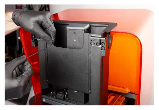
Thread one 2 mm hex screw into each of the four holes. Tighten the screws using the provided 2 mm hex driver. Do not overtighten to avoid stripping the screw threads.
