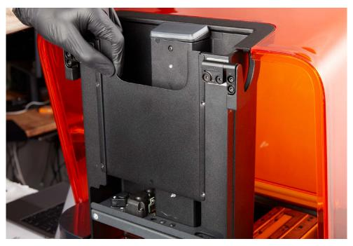
Orient the cartridge slot plate vertically, with the cutout at the top. Align the four holes in the cartridge slot plate with the four screw holes in the Z-tower.
