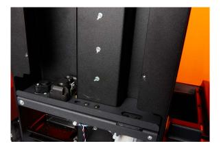
Remove the cartridge slot plate and set it aside.
