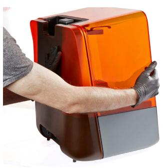
Place the rear shell back onto the printer. Press it towards the front of the printer to ensure that it fully seats in place. There should be no gaps between the rear shell and the side or bottom shells.
