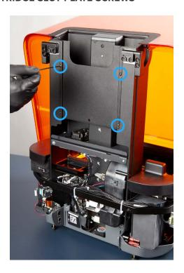
Use the provided 2 mm hex driver to loosen and remove the four screws holding the cartridge slot plate to the Z-tower.
