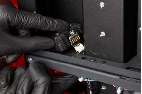
Plug the cable into the cartridge spring finger assembly. The cable will only enter the connector in the correct orientation. Be careful not to bend the pins in the connector.
