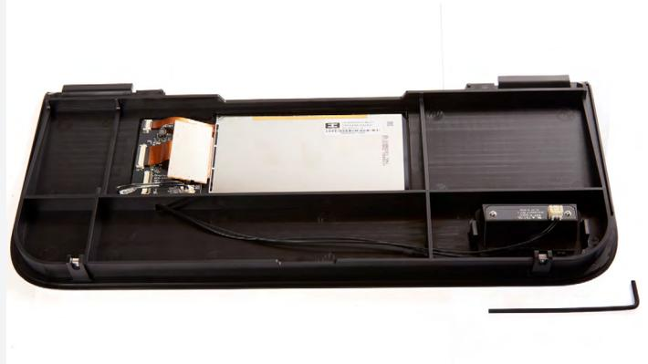
The Form 3 has a touchscreen in its front shell. The touchscreen is the primary means of interacting with and controlling the printer, so a broken or malfunctioning touchscreen can prevent the printer from being used normally.
