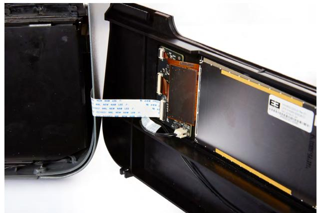
Rotate the latch towards the display assembly to lock the display ribbon cable in place.
