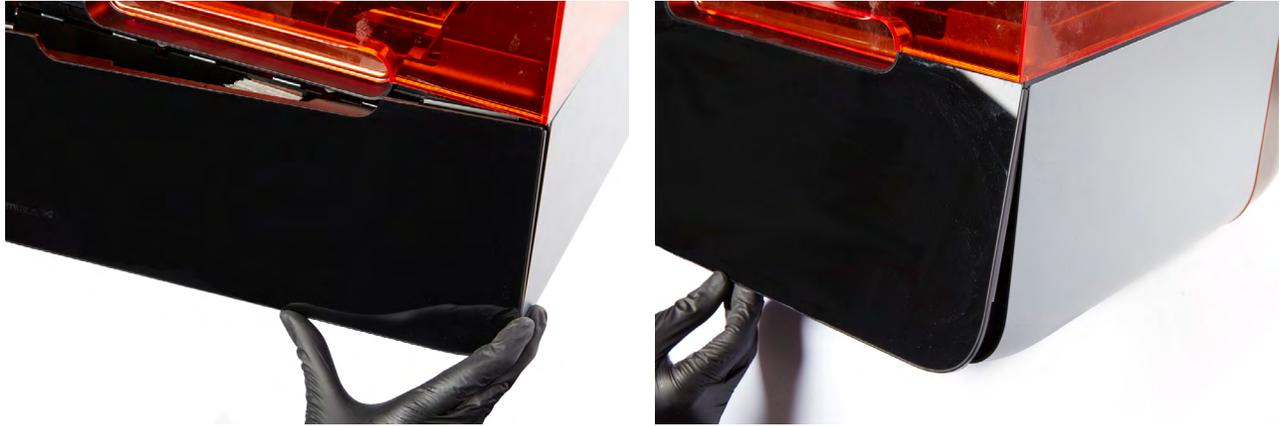
Insert the tabs on the top edge of the display assembly underneath the top shell of the printer. Tilt the bottom edge of the display assembly towards the printer until it lies flush with the bottom shell and side shells. Ensure that the display ribbon cable is not caught between the display assembly and the printer frame.
