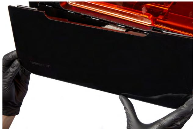
The top of the display assembly is held to the printer frame via a set of plastic tabs. Tilt the bottom of the display assembly slightly away from the printer, then lower the display assembly to separate it from the printer frame.
