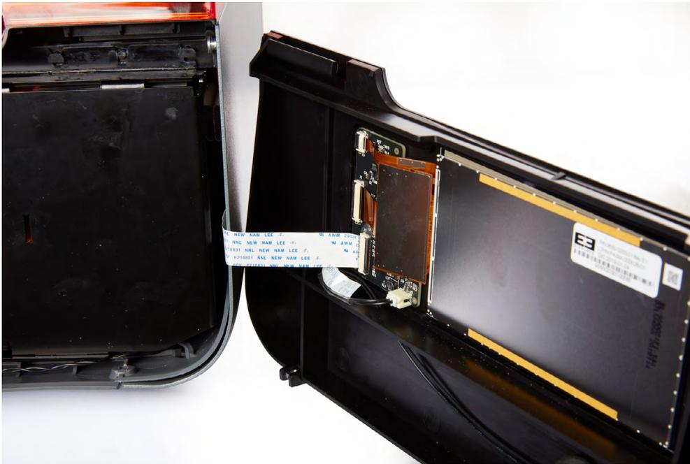
The display ribbon cable connects the display assembly to the printer motherboard. Rotate the display assembly to the right to access the display ribbon cable connector.
