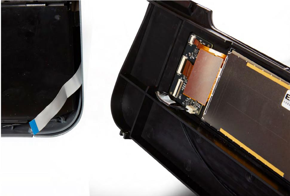
Remove the display ribbon cable from the connector and set the display assembly aside.
